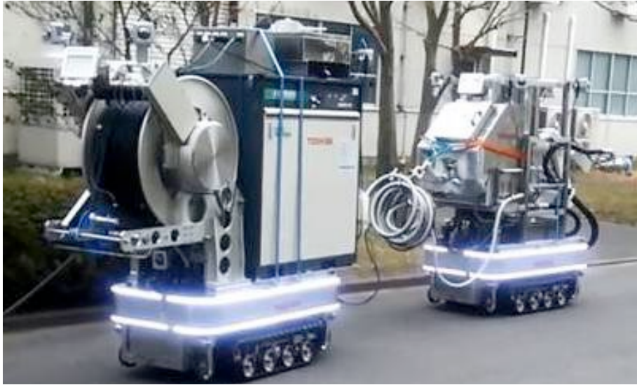
Dry Ice Surface Blaster/Vacuum Robot System
