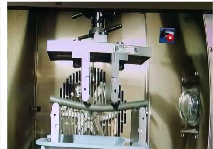
Four-point bend test of 150mm long segment to measure bending modulus
