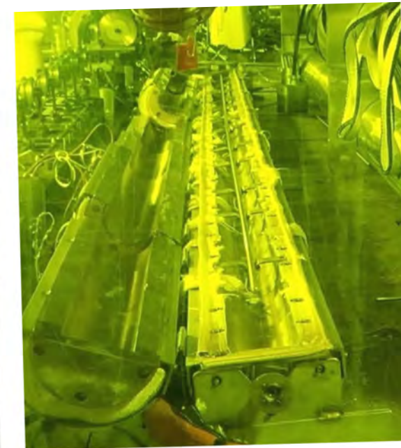
Full-length rod heat treatment oven capable of a variety of temperature profiles
