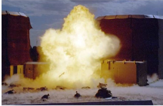
The Dual-Axis Radiographic Hydrodynamic Test Facility (DARHT) uses high-energy pulsed x-rays to test implosion dynamics using non-nuclear components.
