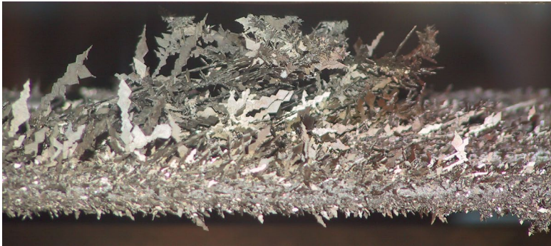
Electroplated uranium from pyroprocessing
