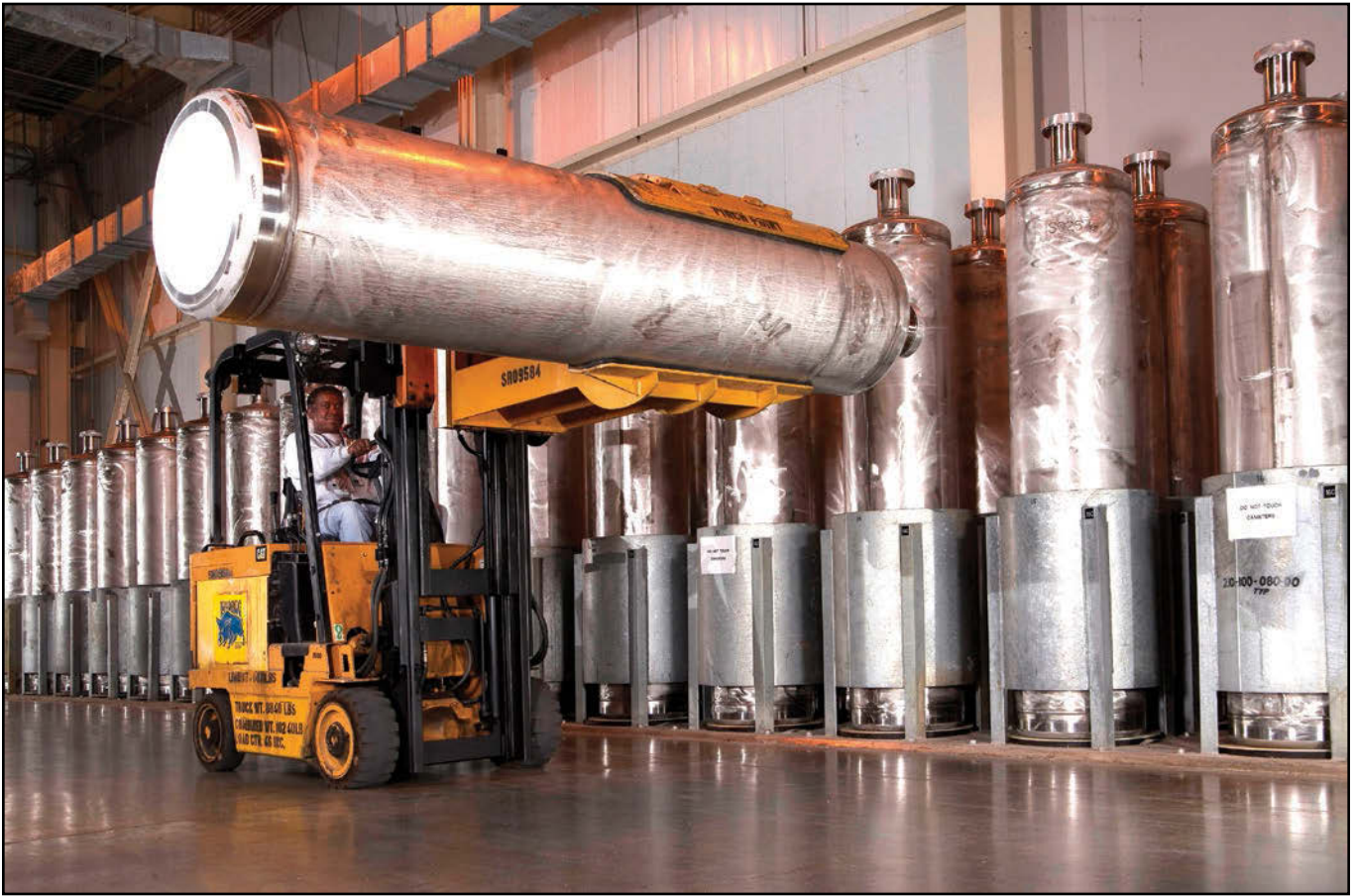
High-activity liquid waste from the waste tanks at SRS goes to the DWPF, where it is vitrified, then stored in these 10-foot-tall stainless steel canisters. A forklift operator transports an empty canister.
