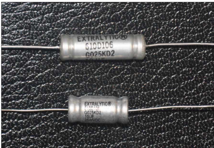
Fig. 4. Comparison of an authentic electrolytic capacitor (top) and a suspected counterfeit/fraudulent capacitor (bottom).
