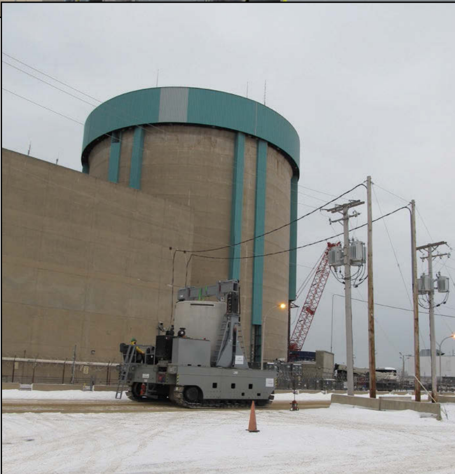
A cask is loaded onto a track-driven cask transporter in preparation of transfer to the Zion ISFSI.
