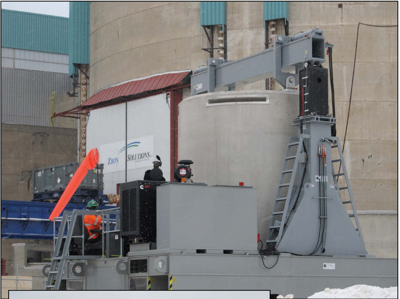
A cask is loaded onto a track-driven cask transporter in preparation of transfer to the Zion ISFSI.
