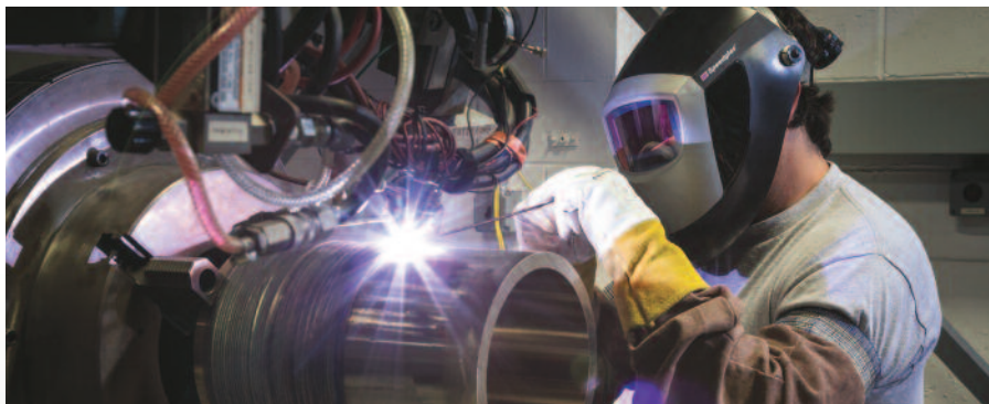
A machine-arch, gas tungsten welding process called hard surfacing is performed on a Stellite™ product at a Westinghouse manufacturing facility.
