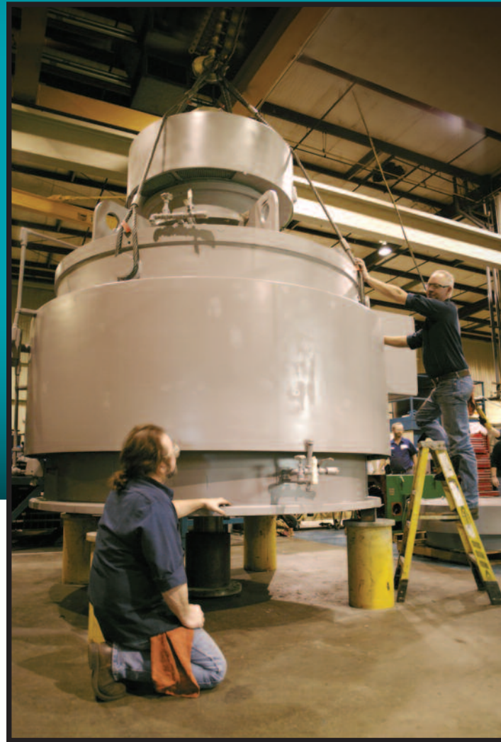
IPS has years of experience repairing safety- and non-safety related nuclear motors up to 13.8 kV and weighing over 93,000 lbs.
