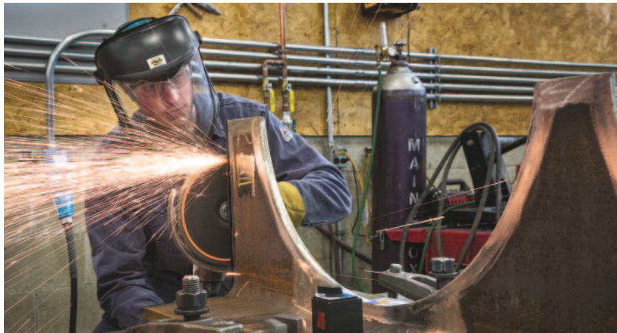
An air tank mid-frame is prepared for fabrication by a Westinghouse fabrication mechanic.
