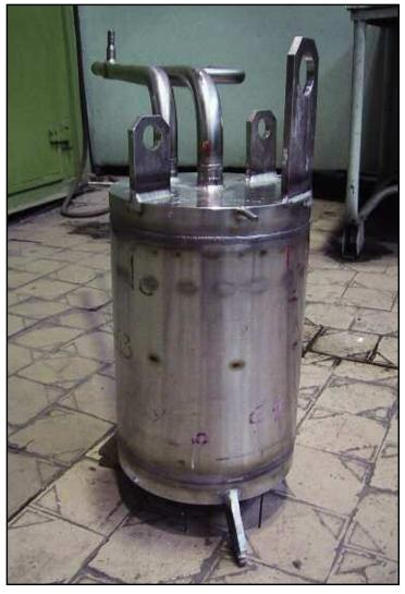
U.S.-Kazakhstan design cesium trap (shown without shielding).
