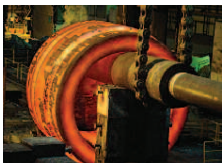
The Reactor Pressure Vessel integrated nozzle shell ingot. Forgings must be ordered many years ahead of time.
