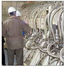
Centrifugal contactors isolate and remove cesium from the salt waste solution stored in waste tanks at Savannah River. The article beginning on page 31 discusses the cesium removal system at the
