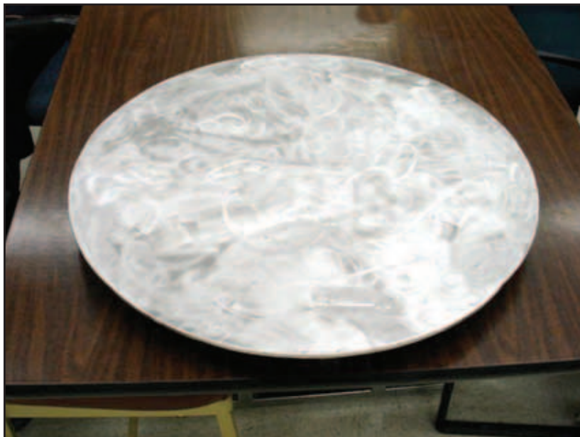
The "lazy susan" allows the position of the waste package to be changed with minimal handling, thereby reducing dose to the fissile material handler.
