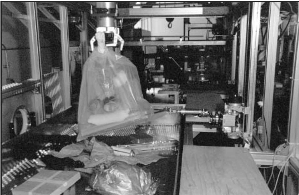
Fig. 3. The gripper, located at the end of the Z-Mast, positions a bag of simulated wastes as pneumatic scissors get ready to cut the bottom of the bag, allowing the contents to drop onto the sorting table.
