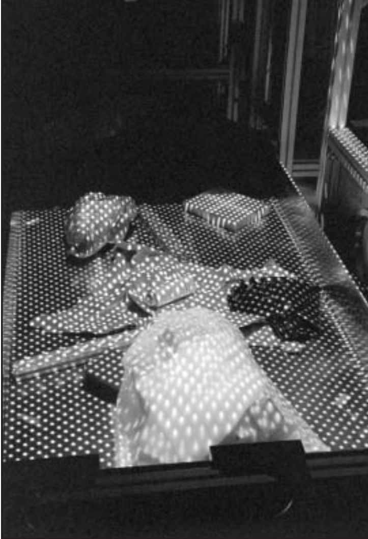
Fig. 4. To provide a three-dimensional profile of table contents, waste items on the sorting table are measured using stereo cameras and projected arrays of light from the StarCam imaging system.
