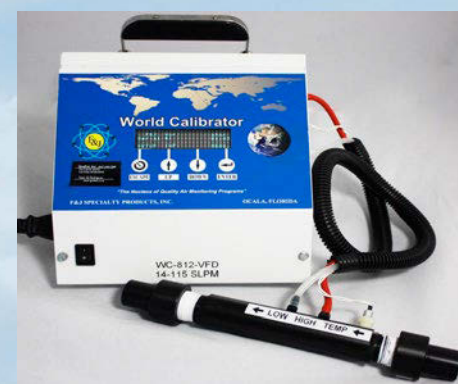
World Calibrator VFD Version ± 1% F.S. Accuracy PC Interfaceable
