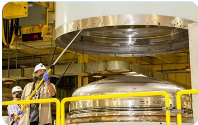
A radiological worker surveys the inside of a TRUPACT-II containment lid during waste handling operations at the Waste Isolation Pilot Plant. (Photo: DOE)
