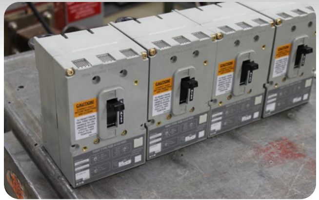
Breaker for dedication, Eaton Navy type: AQB-A103 RMS. An example of a commercial product with high reliability that may be excluded from testing.
