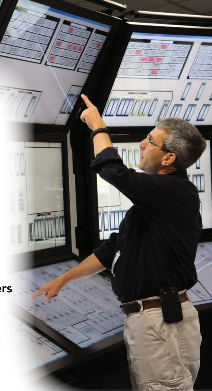
An Idaho National Laboratory simulation lab with panels that can be reconfigured for U.S. nuclear plant control room training and modernization.
