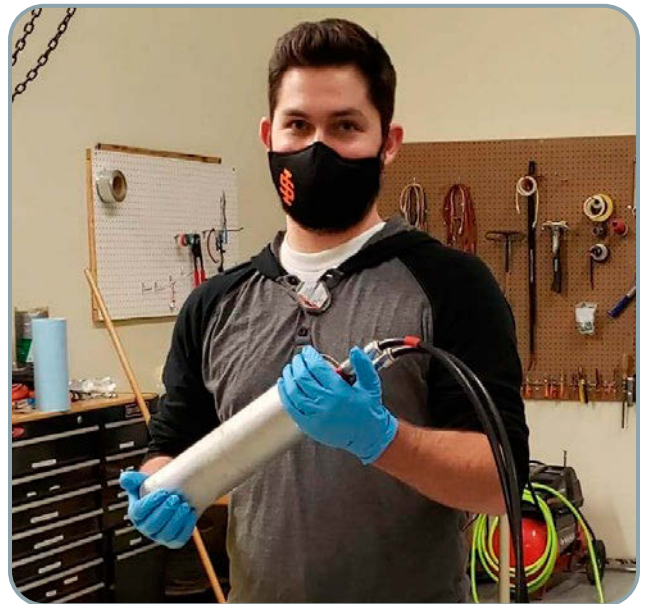
Ercanbrack, holding a boron trifluoride ( \text{BF}_3 ) ionization chamber used to provide reactor neutronics information to safety channel number 2 on the reactor control console. The ionization chamber was removed from the reactor to undergo tests.
