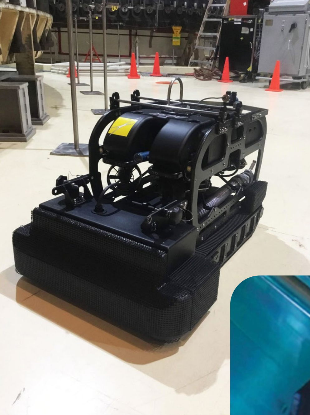
A decontamination ROV on a dry surface and in action in a refueling cavity.
