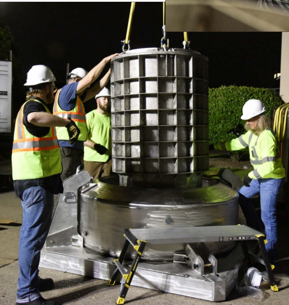
An NNSA team uses a 435-B Type B container to recover a cesium-137 self-shielded irradiator from a hospital in Houston. (Photo: NNSA)
