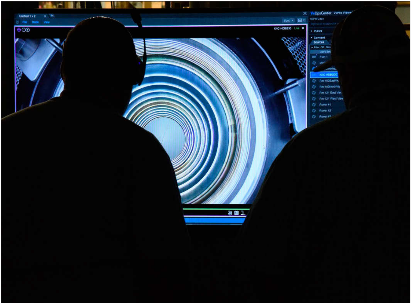
Workers examine a video screen showing the interior of the Multi-Mission Radioisotope Thermoelectric Generator prior to fueling.
