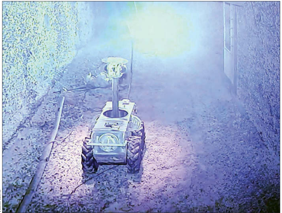
SRNL's tethered robotic crawler inspects the H Canyon exhaust tunnel at SRS in 2019.
