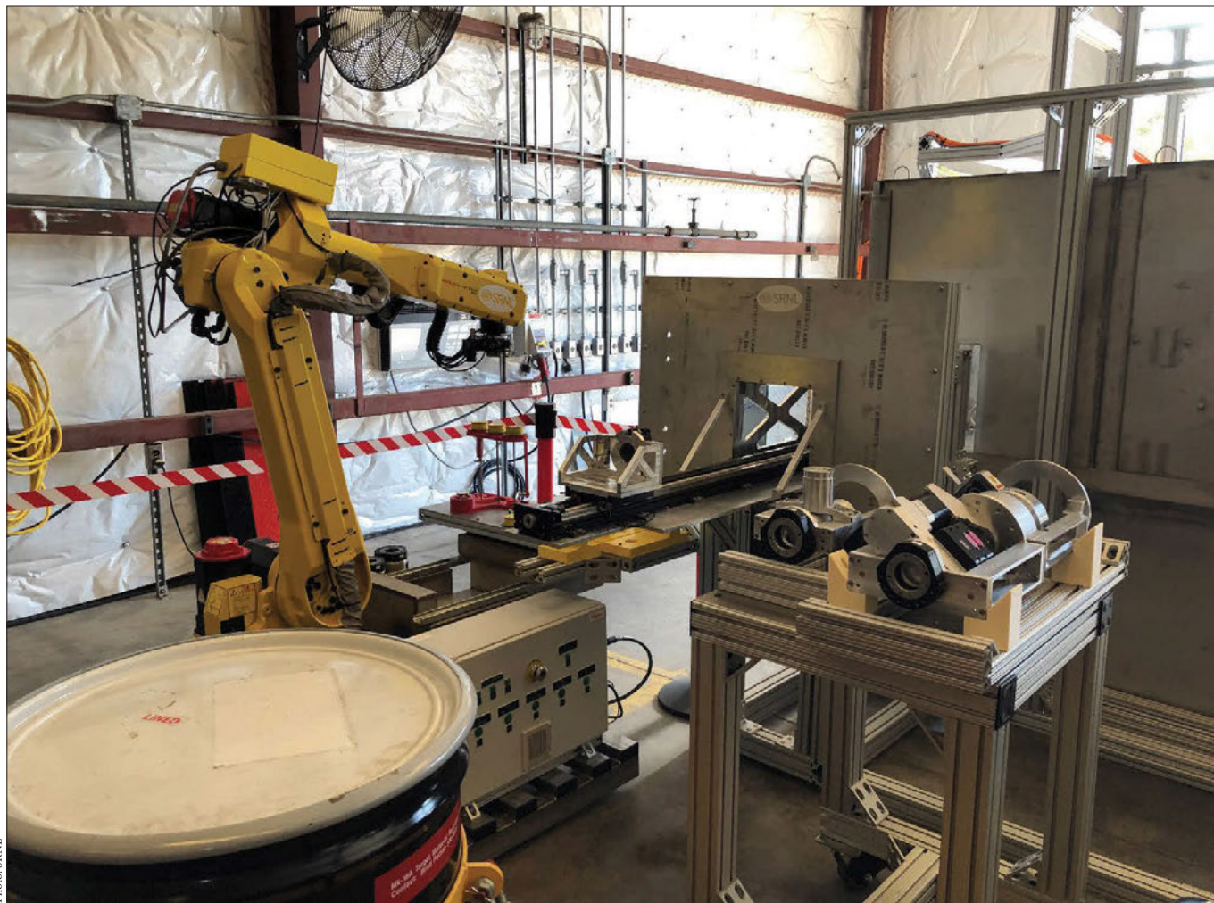
A robotic arm adapted by SRNL for the Pu-244 recovery campaign with associated equipment in the mock-up facility at SRS.
