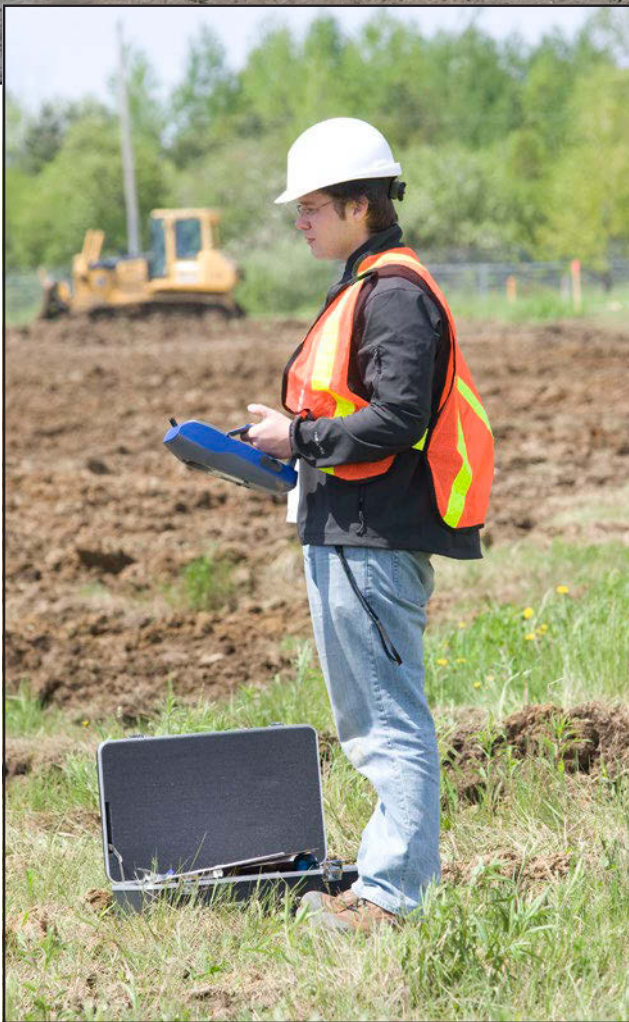
Dust monitoring is ongoing whenever PHAI construction is underway. The PHAI dust management plan sets out limits and action levels to ensure that dust is controlled and mitigated on-site for the protection of people and the environment.
