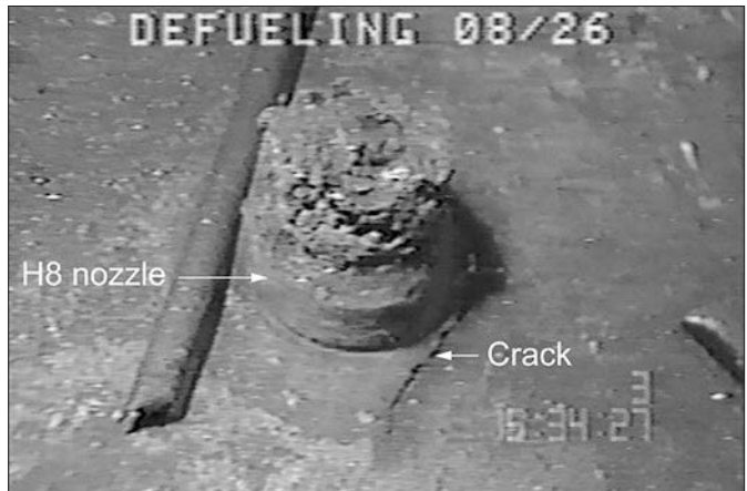
Fig. 1. TMI-2 video examinations revealed locations where damage to the core barrel (left) and nozzles (right) was more severe.
