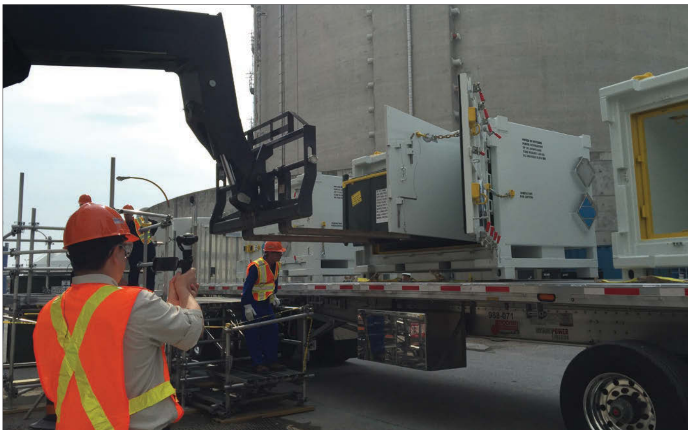
A low-level waste container is placed inside a shielded container for shipment to a licensed facility for storage.
