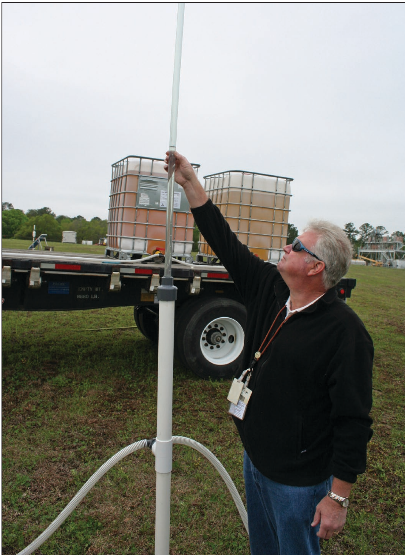
SRNS engineering and technical support specialist Keith Hyde measures the flow of vegetable oil during an injection process that greatly increases the underground population of naturally occurring chemical-eating bacteria at SRS.
