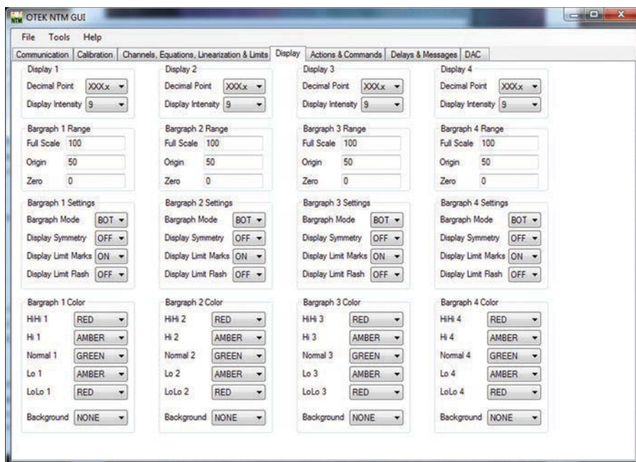
Fig. 2. A screen shot of Otek’s user software interface displaying the NTM meter configuration settings
