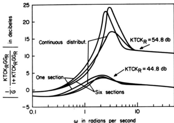
FIG. 8. Attenuation characteristics of the closed-loop transfer function  $[(1/G)KTCK_R GG_R / (1 + KTCK_R GG_R)]$
