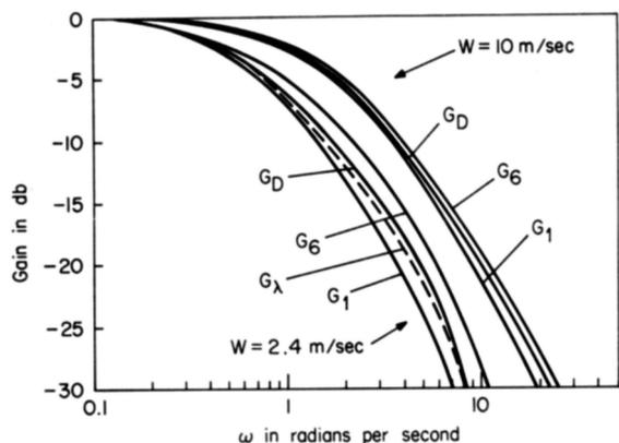
FIG. 2. Attenuation characteristics of the power-coolant temperature transfer functions
