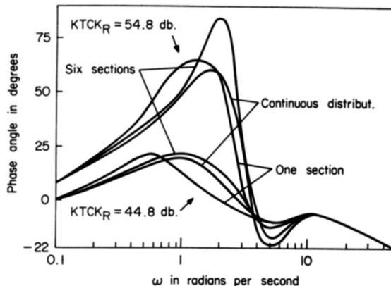
FIG. 9. Phase angle characteristics of the closed-loop transfer function  $[(1/G)KTCK_R GG_R / (1 + KTCK_R GG_R)]$
