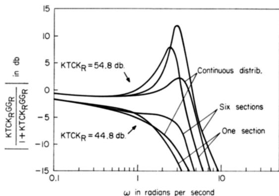
FIG. 6. Attenuation characteristics of the closed-loop transfer function  $[KTCK_R GG_R / (1 + KTCK_R GG_R)]$
