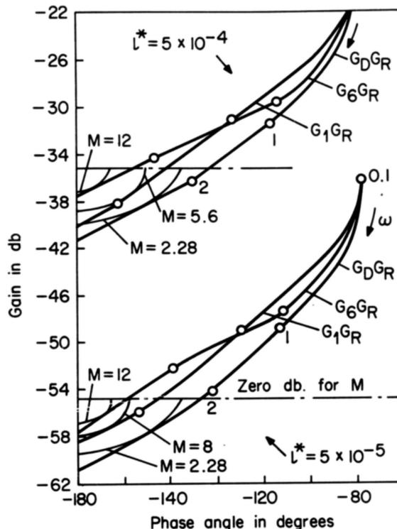
FIG. 4. Open-loop transfer functions of reactor internal loop ( $w = 2.4$  meters/sec)
