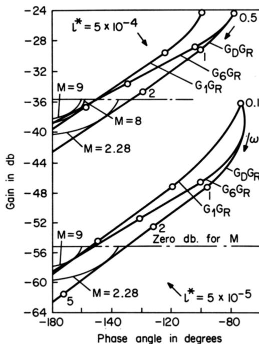
FIG. 5. Open loop transfer functions of reactor internal loop ( $w = 10$  meters/sec)
