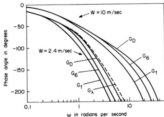
FIG. 3. Phase angle characteristics of the power-coolant temperature transfer functions
