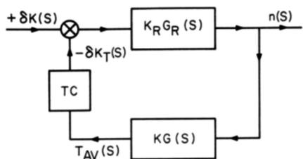
FIG. 1. Reactor internal feedback loop
