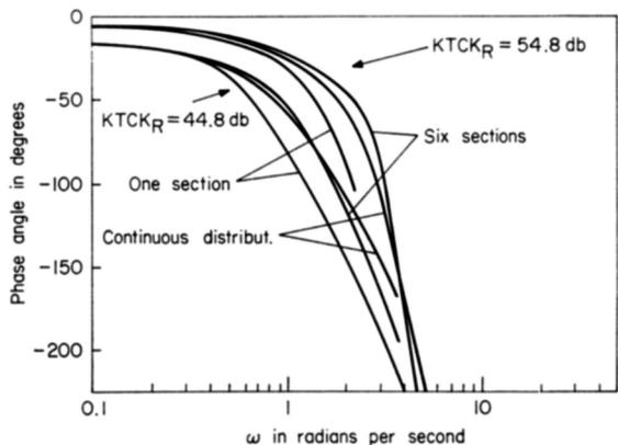
FIG. 7. Phase angle characteristics of the closed-loop transfer function  $[KTCK_R GG_R / (1 + KTCK_R GG_R)]$
