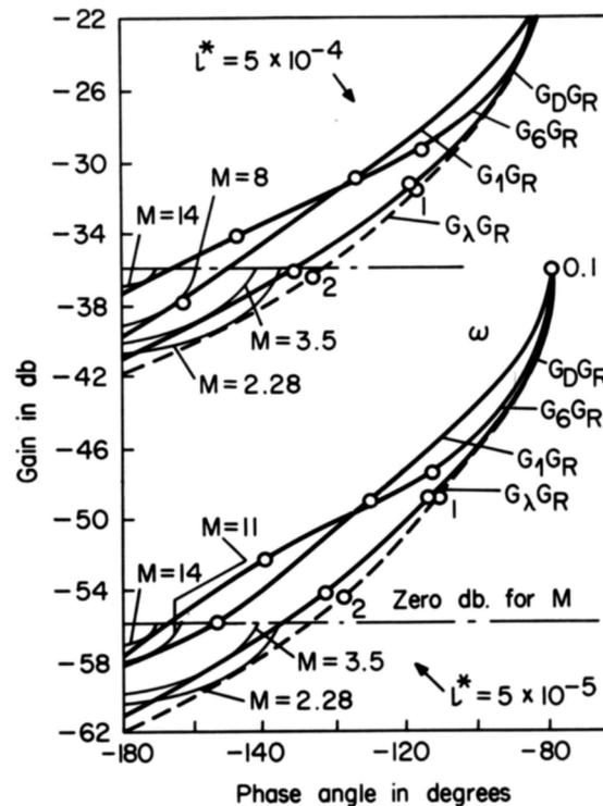
FIG. 10. Open-loop transfer functions of reactor internal feedback loop
