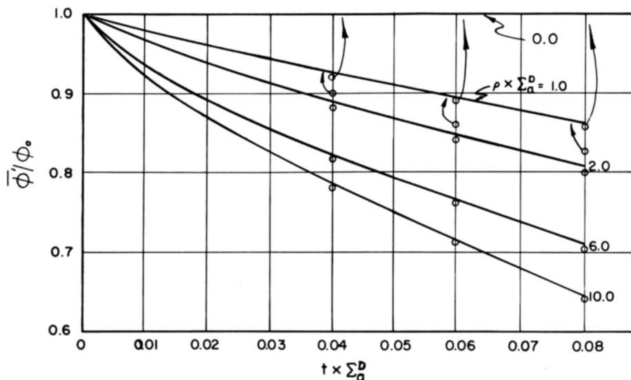
FIG. 1. The average normalized scalar flux in a coin-shaped detector in water for various radii  $\rho$  and thicknesses as calculated by the variational and the integral methods.  $\circ$  variational method; — integral method.
