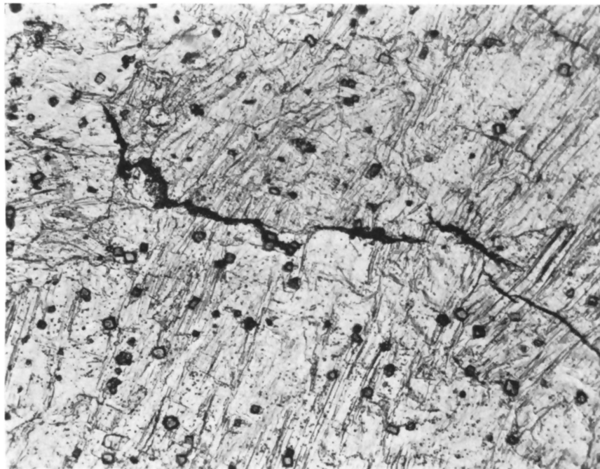
FIG. 2. Photomicrograph of cluster fuel element irradiation to 2200 MWD/T. Maximum temperature \sim 520 (t). Cathode etch at 250X (bright field).
