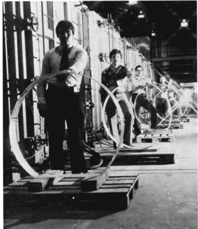
Fig. 7. Borosilicate glass blanks for the Nova turning mirrors.
