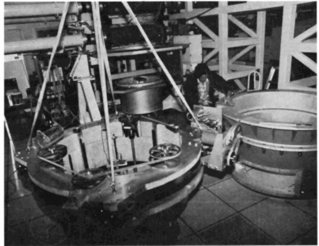
Fig. 16. Focus lens drive mechanism in final assembly.
