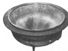
Boral-lined neutron shielding jacket
