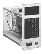
SCALERS. With or without preset count in count capacities from 10<sup>1</sup> to 10<sup>12</sup>. Accept pulse inputs to 10 mc/sec continuous with pulse-pair resolution less than 10 nanoseconds.
