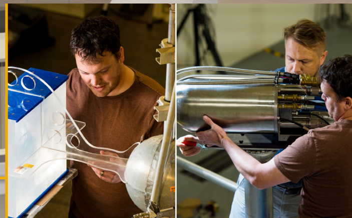
Setup for Moderated ^{252}\text{Cf} Irradiation (left), D-T Neutron Generator (right)
