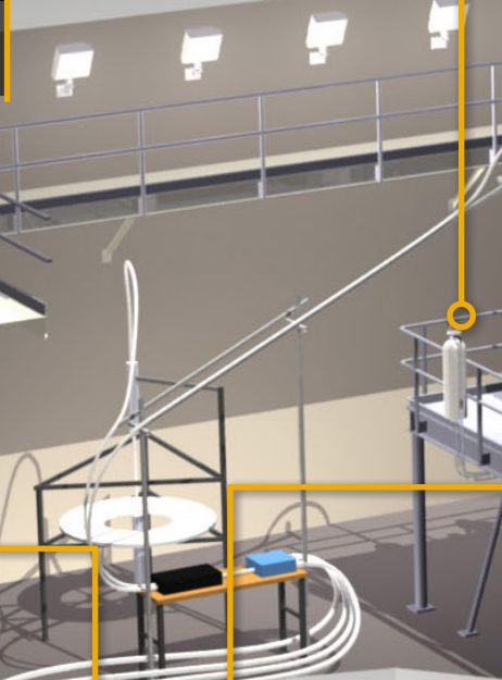
Setup for Moderated ^{252}\text{Cf} Irradiation (left), D-T Neutron Generator (right)
