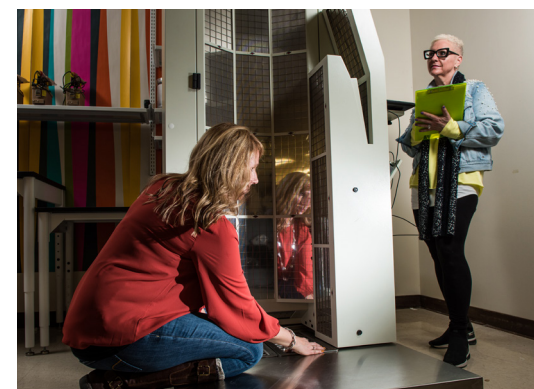
PNNL staff support nuclear worker protection by testing and calibrating personal contamination monitors.
