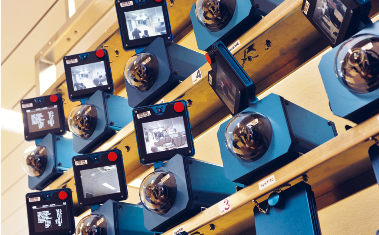
Next Generation Surveillance System (NGSS) Cameras installed at the Department of Safeguards' laboratories for testing prior to installation in nuclear facilities.
