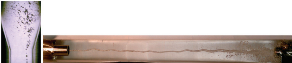
Fig. 1 the components of gas extraction system: 1. bubble generator, 2. bubble separator
