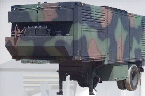
MEP-810: deployable diesel power generation.
