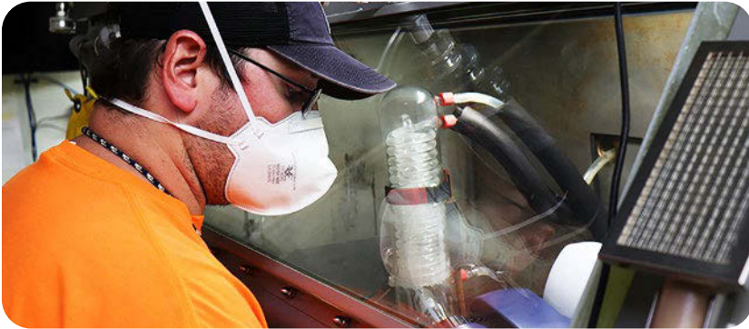
A fissile material handler uses a shielded glovebox to dissolve U-233 into a low-level form so that it can be mixed with grout for safe transportation and disposal. Photo: DOE
