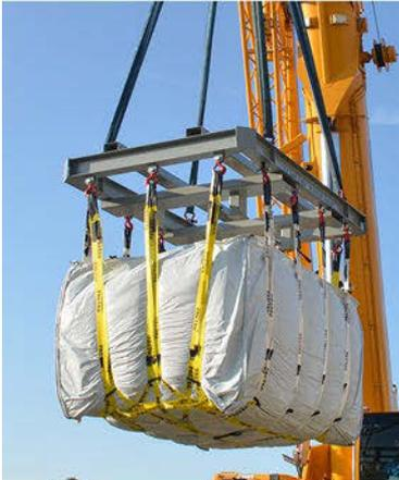
PacTec's 7A Type A / IP-3 LiftPac® is designed and tested for the shipment, storage and disposal of D&D debris and other flowable solids such as GAC, soil and gravel.
