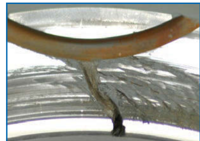
Face seal damage (above) caused by electrostatic erosion. AEGIS® RPPR (below) installed on a reactor recirculating pump.
