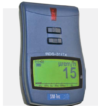
RDS-31 TD™ Multi-purpose Survey Meter Training Device
